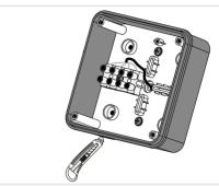
Connect the power cord wires to the terminal block and assemble the fan in reverse order. Supply power to the fan.
