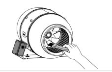
Connect an air duct on both sides of the fan. Supply power to the fan.
