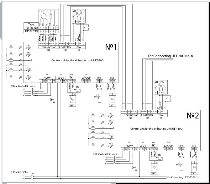
Fig. 11. Schematic Diagram for Connecting Several UET-30D Control Units
