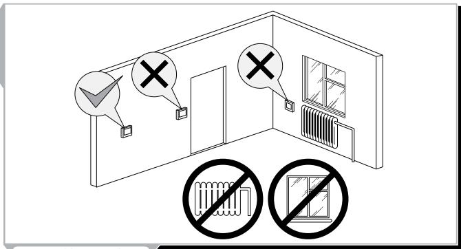
Fig. 5. Digital Thermostat Installation
