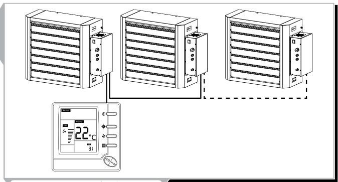
Fig. 10. Series Connection of Several Units
