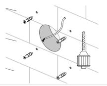
Connect the fan to the electric mains according to the connections diagram. Install the front panel by turning it clockwise. Thread the fixing screw.
