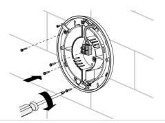
The fan delivery set includes a specially designed plastic screwdriver for fan settings adjustments.
