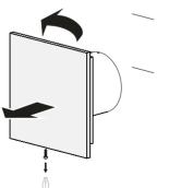
Mark the holes for fixing the fan and the power cable.
