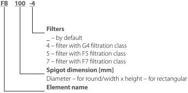
FB – filter with a flat filter element
