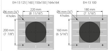
3. Insert the supplied expansion anchors 6 mm ( $\frac{1}{4}$ )x40 mm ( $\frac{19}{16}$ ) into the holes.
