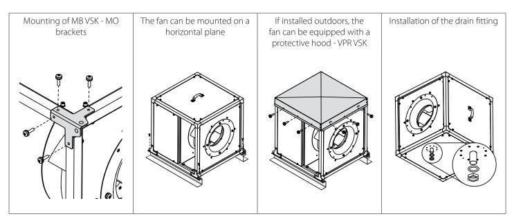
The MK VSK brackets and the VPR VSK protective hood are not included in the delivery set and must be ordered separately.
