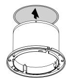
4. Install the front grille on the diffuser by turning it clockwise until the bayonet connection clicks.
