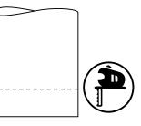
3. Secure the diffuser to the ceiling using wall plugs and/or selftapping screws depending on the ceiling material.
