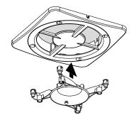
8. If it is necessary to adjust the air flow, install a throttle (air flow regulator) in the diffuser by removing the inserts from it until the required air flow is reached (only for F4 125 FBR; for F4 125 FB, the throttle is not included in the delivery set, must be ordered separately).
