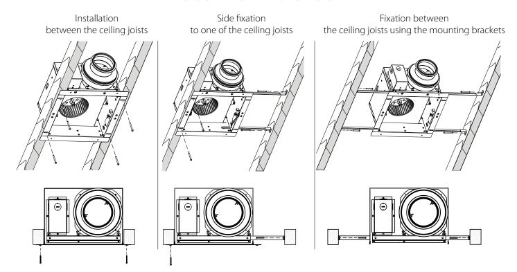
Additional fastening holes in the fan casing may be used for mounting purposes
