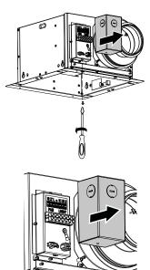
Remove the protective cap and install the cable gland.
