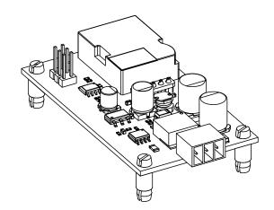
Install the sensor circuit board inside the unit in the bracket holes or in the wall at location specified in the user manual.
