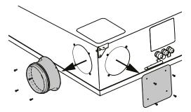
Then mount the spigot in place of the plug and the plug in place of the spigot.
