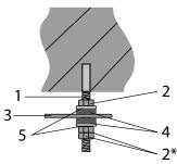
Fixing through a suspended ceiling
