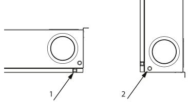
Location of the drain pipe for suspended (1) and wall-mounted (2) units
