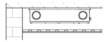
WARNING! Wall mounting of the units is only possible with the drain pipes facing downwards.
