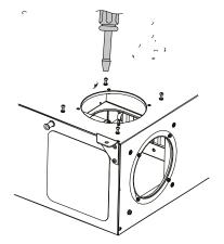
WARNING! Before starting installation work, areas with plugs and around pipe openings inside the unit must be covered with appropriate insulating pads (included in delivery kit).
