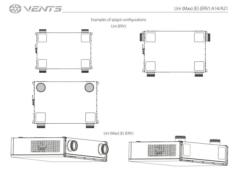
The Uni (Max) (E) (ERV) units are equipped with air dampers. When changing the spigot position, it is necessary to reinstall the corresponding damper.
