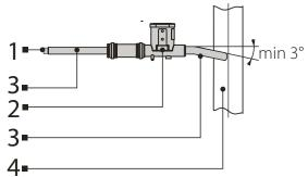
1 - drain pipe of the unit; 2 - U-trap; 3 - connecting pipe; 4 - sewage system.
