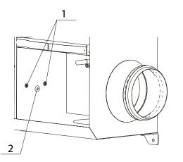
1 — threaded rivet for fixing the sensor
