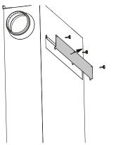
The unit is equipped with a service panel for connection and maintenance.
