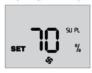
To restore factory settings, enter the Fan Speed Setting mode, synchronously press and hold  $\triangle$  and  $\bigcirc$  for 3 seconds.
