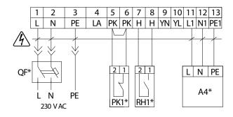
Connection of additional external control contacts is implemented in the control unit. For accessing the control unit open the unit door, release the screws fixing the shielding and remove it.
