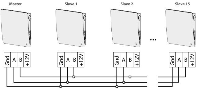
WARNING! Never connect + 12V power lines from multiple devices!
