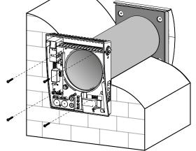
8. Route the power cable as figured below and connect the ventilator to power mains in compliance with the external wiring diagram, see section **Connection to power mains**. Secure the power cable with the clamp.
