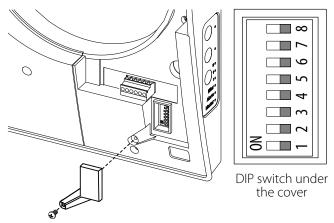
Prior to operating the ventilator set its operation modes using the DIP switch. It is located on the controller circuit board. To access the DIP switch, take off the front panel of the indoor unit and uplift the rubber plug that covers the switch.
