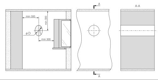
2. Insert the air duct in the wall. For ease of installation use the mounting wedges included in the delivery set.
