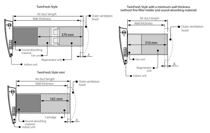
If the wall thickness is less than that in the layout of the blocks inside the wall, you can unfasten the fine filter holder and assemble the ventilator without it and without sound-absorbing material, as shown in the figure above.
