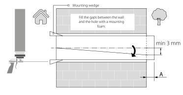
Install the air duct with the minimum slope of 3 mm downwards from the outer wall side.
