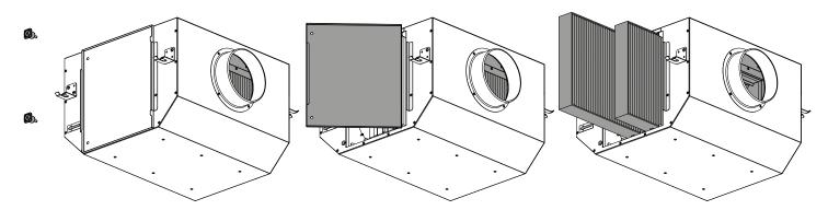
The technical maintenance of the electrostatic filter includes periodic cleaning of the surfaces from accumulated dust and dirt. Clean the electrostatic filter with a soft brush or a vacuum cleaner.
