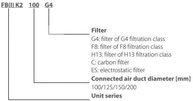
FB K2: filter box with panel filters for round air ducts
