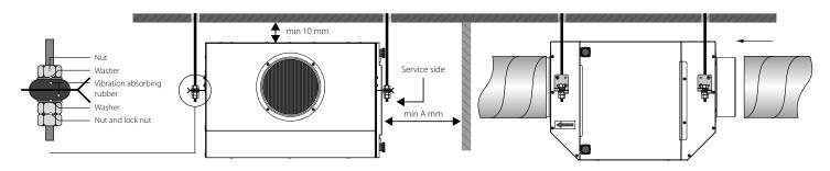
To get the best performance of the ventilation system and to minimize turbulence-induced air pressure losses, connect the straight air duct section to the spigots on both sides of the unit while installing.
