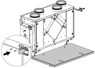
Service side change is shown by the example of the VUT/VUE 300 V2 mini EC air handling unit. The procedure of the service side changing for the VUT/VUE 300 H2 mini EC unit is carried out in the same manner.
