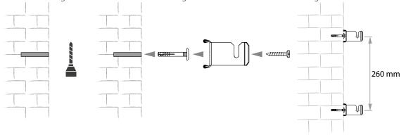
3. Install the unit on the mounting brackets. Tighten the triangular fixing screws on the mounting brackets.
