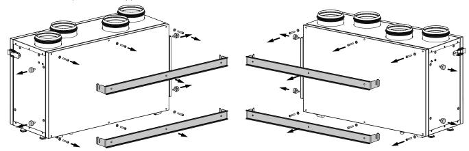
3. Install the latches and the service panel on the opposite side of the unit.
