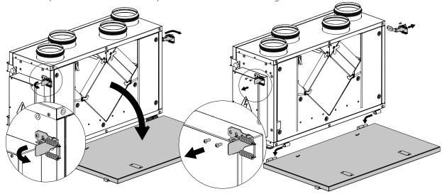
2. Remove four hand screws and take off the suspension brackets. Then unscrew six fixing screws from the back panel and remove the panel. Install the back panel on the opposite side of the unit.
