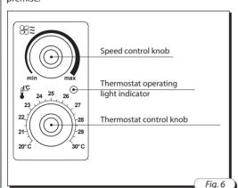
The front panel of the electronic module has the following controls and indicators:
