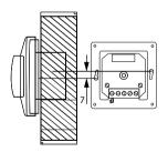
The controller should be installed on a vertical wall indoors in a hidden mounting box. Inspect the unit visually and check the casing for integrity.
