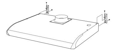
The exhaust is mounted under or inside a kitchen cabinet. The unit also allows console mounting with the optional accessories purchased separately.
