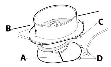
Mount the flange with the valve **A** to the exhaust opening of the kitchen hood. Make sure that flange **B** detents catch against the underside surface adjacent to the hole and then secure it with latches **C** in holes **D**.
