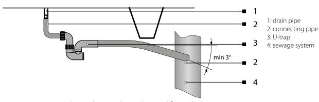
Prior to starting operation make sure that water has unobstructed flow in the sewage system. Fill the U-trap with water before operation.
