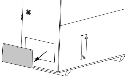
To change positioning of the air ducts use the plugs from the side walls for the front panel.
