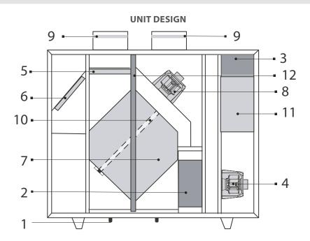
1: drain pipe; 2: water heater (only for the units with water heater); 3: electric heater (only for the units with electric heater); 4: supply fan; 5: supply filter; 6: extract filter; 7: heat exchanger; 8: extract fan; 9: air flow control damper with electric actuator; 10: bypass damper; 11: control unit; 12: removable holder
