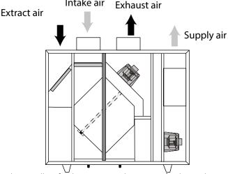
Connection of the air ducts is shown with the stickers of the respective colours: yellow for the extract air duct, green for the intake air duct, red for the supply air duct and brown for the exhaust air duct.
