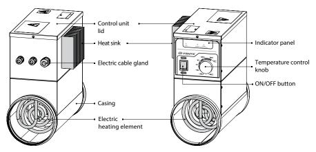
The NK...U heaters with integral control units for rectangular ducts consist of a casing with a rigidly mounted junction box. The junction box has a removable front panel featuring the temperature control knob, the ON/OFF button and the indicator panel.
