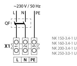
Wiring diagram of NK...U with capacity from 3.0 kW to 9.0 kW with a control unit for round ducts and with capacity 4.5 kW to 54 kW for rectangular ducts (whole model range)
