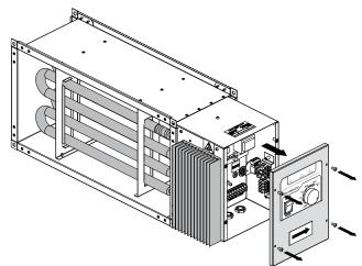
Connection of NK...U(Un) with capacity from 0.6 to 2.4 kW with integrated temperature control module for round air ducts
