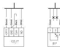
Connecting humidity sensor or  ${\rm CO}_2$  sensor to the control unit via a cable, which is attached to the bracket
