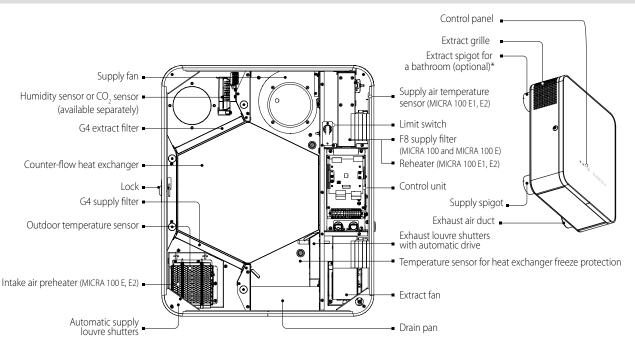
Warm stale extract air from the room flows to the unit, where it is filtered by the extract filter, then air flows through the heat exchanger and is exhausted outside by the extract fan.
