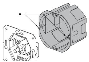
3. Insert the mounting box in the wall. The cable from the delivery set may be replaced with a cable of required length, type 3x0.5 mm<sup>2</sup> and max. length of 10 m.
