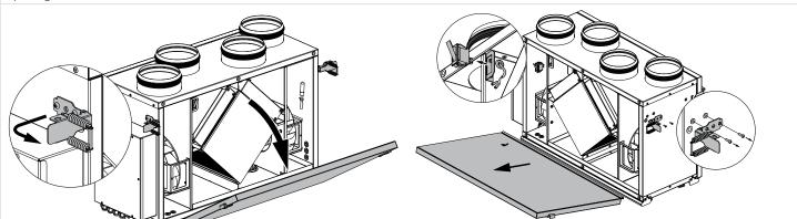
2. Remove four triangular screws and suspend the suspension brackets. Then unscrew six fixing screws from the back panel and remove the panel. Install the back panel on the opposite side of the unit.
