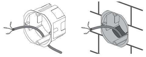
4. Connect the cable to the speed controller following the wiring diagram on page 15. Install the speed controller inside the mounting box using screws.
