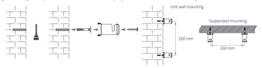
3. Install the unit on the mounting brackets. Tighten the triangular fixing screws on the mounting brackets.
