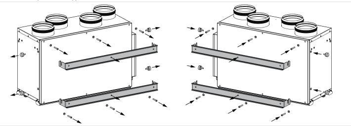
3. Install the limit switch, the latches and the service panel on the opposite side of the unit.
