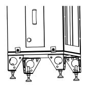
For floor mounting, the feet must be screwed to the heat exchanger.
