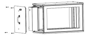
To connect the heat exchanger to the unit, remove the front panel and remove the heating/cooling unit.
