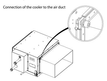
Outdoor installation of the cooler is allowed only if the refrigerant is an antifreeze (ethylene glycol solution). During mounting consider the operating characteristics of the mixing unit actuator.
