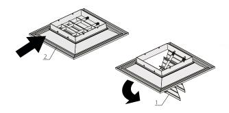
Install the outer frame of the DP diffuser (position 2) on the rail frame from the inside on the edges of a T-profile.
