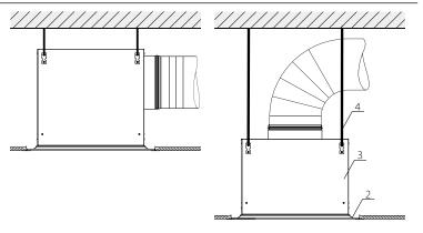
The plenum box (position 3) must be initially secured at a distance of at least 30 cm from the ceiling plane.
