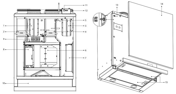
1 — supply fan; 2 — supply filter; 3 — exhaust fan; 4 — exhaust filter; 5 — humidity sensor (optional); 6 — rotary heat exchanger; 7 — control unit; 8 — rotary heat exchanger drive; 9 — electric heater (models equipped with a heater); 10 — cooker hood; 11 — Setup Mode button; 12 — airtight lead-ins; 13 — service panel, 14 — decorative panel (accessory, not included in the delivery set); 15 — cooker hood filters.
