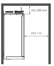
To attain the best performance of the unit and to minimise turbulence-induced air pressure losses connect straight air duct sections to the unit spigots.
