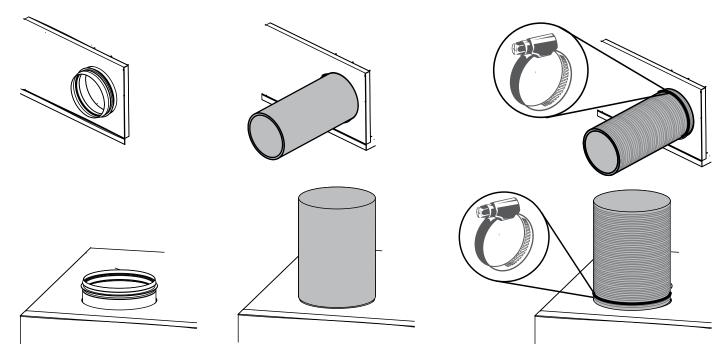
If there are no air ducts or the air ducts are short, it is necessary to protect internal unit parts from ingress of foreign objects at one or more unit spigots. To prevent uncontrollable access to the fan the spigots may be covered with a protecting grille or other protecting device with mesh width not more than 12.5 mm.
