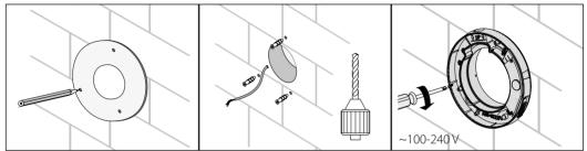
5. Run the power supply cable through the cable gland in the selected way and connect the fan to the power mains as shown in the wiring diagram.
