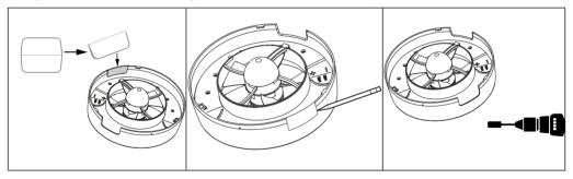
WARNING! Use a power tool with an abrasive attachment or a suitable hand tool to cut the hole.
