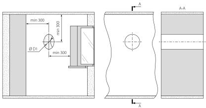
2. Install the telescopic air duct in the hole in such a way that its sections coincide with the outer and inner surface of the wall. For ease of installation, use mounting wedges.
