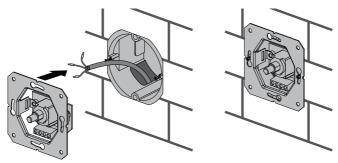
5. Install the front panel of the speed controller as follows: install the front panel, fix the front panel using a washer and a nut, fix the control knob.
