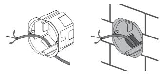
4. Connect the cable to the speed controller in compliance with the wiring diagram. Insert the speed controller in the mounting box using the self-tapping screws.
