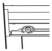
Remove the butterfly bolts that fix the retaining clamp.
