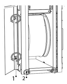
Remove the heat exchangers from the unit. The exchanger block is partially removable for maintenance purposes.
