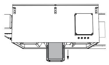
To pull the heat exchanger completely from the unit, open the service door and remove the retaining screws.
