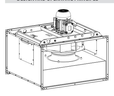
The fan casing is made of galvanized steel.
