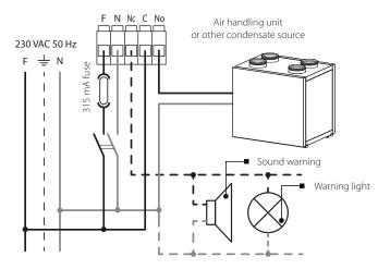
The DN-2 pump is equipped with a C - NO / NC bridging contact (switched current 16 A/250 V AC)
