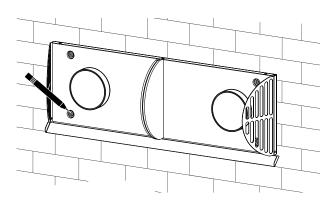
4. Insert the supplied expansion anchors 6x40 into the holes. Fix the back part of the hood on the wall using the supplied screws 4x40.
