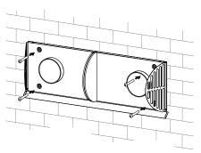
5. Place the front part of the hood on the back part and secure with screws.
