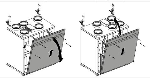
4. Move the service panel to the opposite side, connect it using the ground cable and install in the reverse order.
