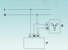
Controller wiring diagram
