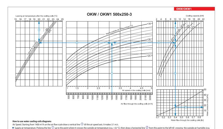
Cooling capacity. Prolong the line up to the point where it crosses the outside air temperature (e.g. +32 °C) and draw a horizontal line from this point to the right until it crosses the outside air humidity curve
