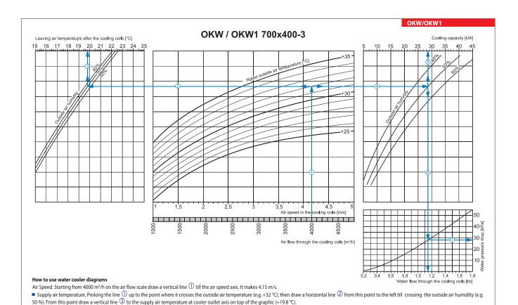
Cooling capacity. Prolong the line 🛈 up to the point where it crosses the outside air temperature (e.g. +32 °C) and draw a horizontal line ④ from this point to the right until it crosses the outside air humidity curve
