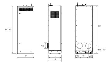
\* The unit height may be adjusted by means of levelling feet.
