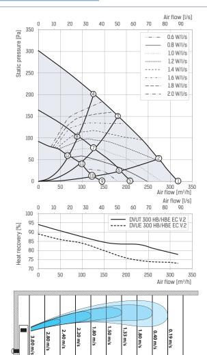
Fresh air stream length produced by DVUT 300 HB EC V.2
