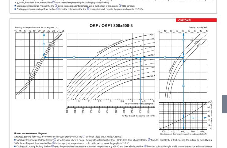
(e.g., 50 %), from here draw a vertical line (5) up to the scale representing the cooling capacity (25.5 kW).
