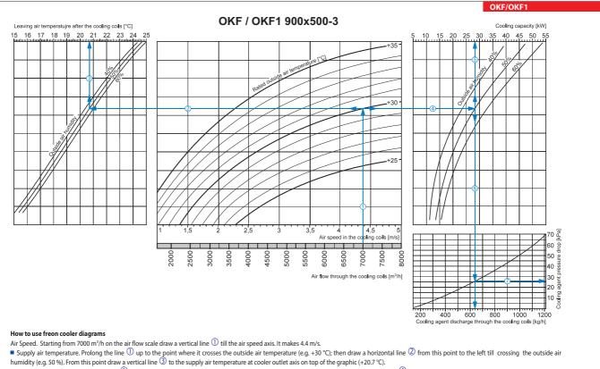
■ Cooling coil capacity. Prolong the line ① up to the point where it crosses the outside air temperature (e.g. +30 °C) and draw a horizontal line ④ from this point to the right until it crosses the outside air humidity curve (e.g., 50 %), from here draw a vertical line (5) up to the scale representing the cooling capacity (28.0 kW).
