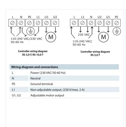
Controller wiring diagram
