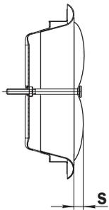
The internal part of the air disk valve is pulled out to ensure the required clearance S (mm) to provide required air flow according to the diagram.
