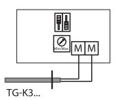
Connection of the sensor for maximum temperature
