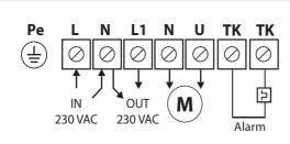
Controller wiring diagram
