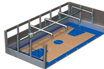
VS fan gym ventilation example
